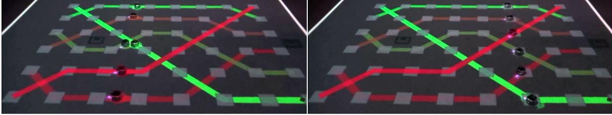
(a) The controller is *collision-free* – robots get as close as  $\delta$ . (b) Braid points are reached simultaneously.
